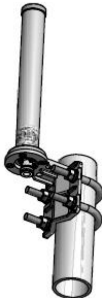
Fig 3. Antenna mounted to the POLE END ONLY.
